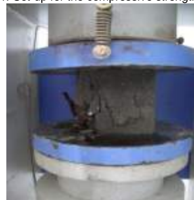
Fig. 1. Set-up for the compressive strength test.
