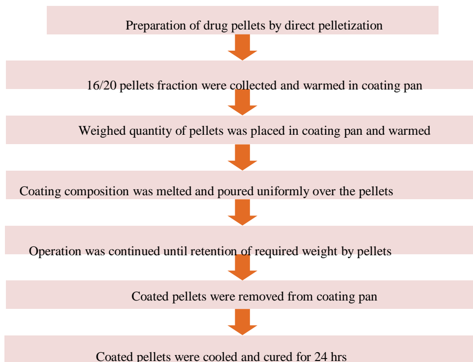
Figure-1: Schematic representation of preparation of HMC pellets of ofloxacin.
