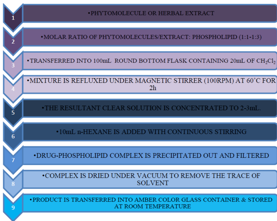
Fig. (2). Formulation schematics of phospholipid complex of phytopharmaceuticals. (A higher resolution / colour version of this figure is available in the electronic copy of the article).
