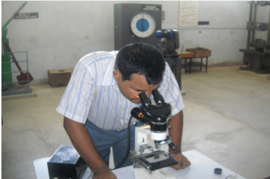
Figure 1: Measurement Of Weld Bead Dimensions With Metallurgical Microscope
